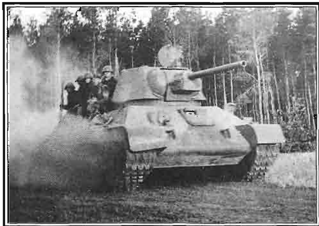
Above: Trying to avoid breathing in the dust thrown up by its tracks, infantrymen ride on a T-34 which is making its way out to the front lines. Handholds were provided on later Soviet tank models.
