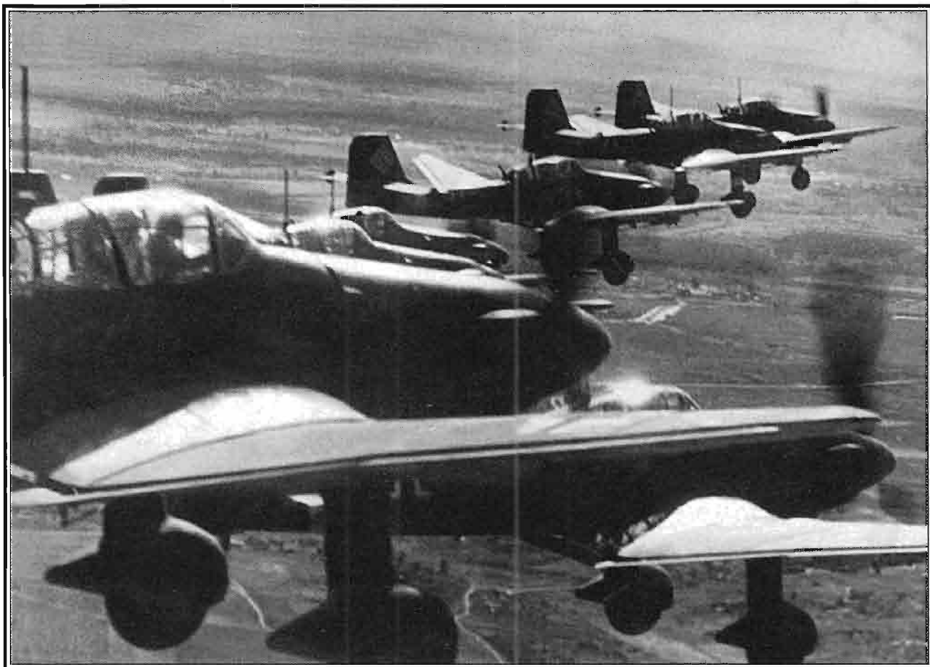
Above: Even though they were particularly vulnerable to enemy fighters due to their slow speed, Stukas were successfully used as anti-tank aircraft when fitted with a 37mm (1.47in) gun under each wing.
